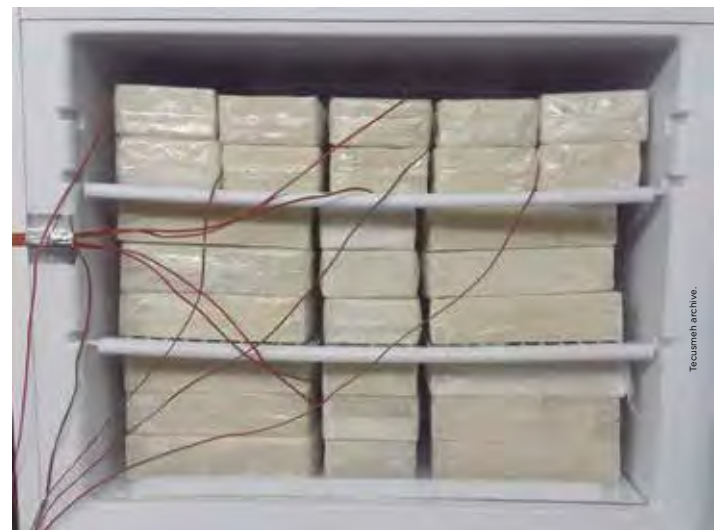
The figures above belong to the freezer compartment of a fully loaded duplex refrigerator for carrying out storage, consumption and temperature rise tests.
