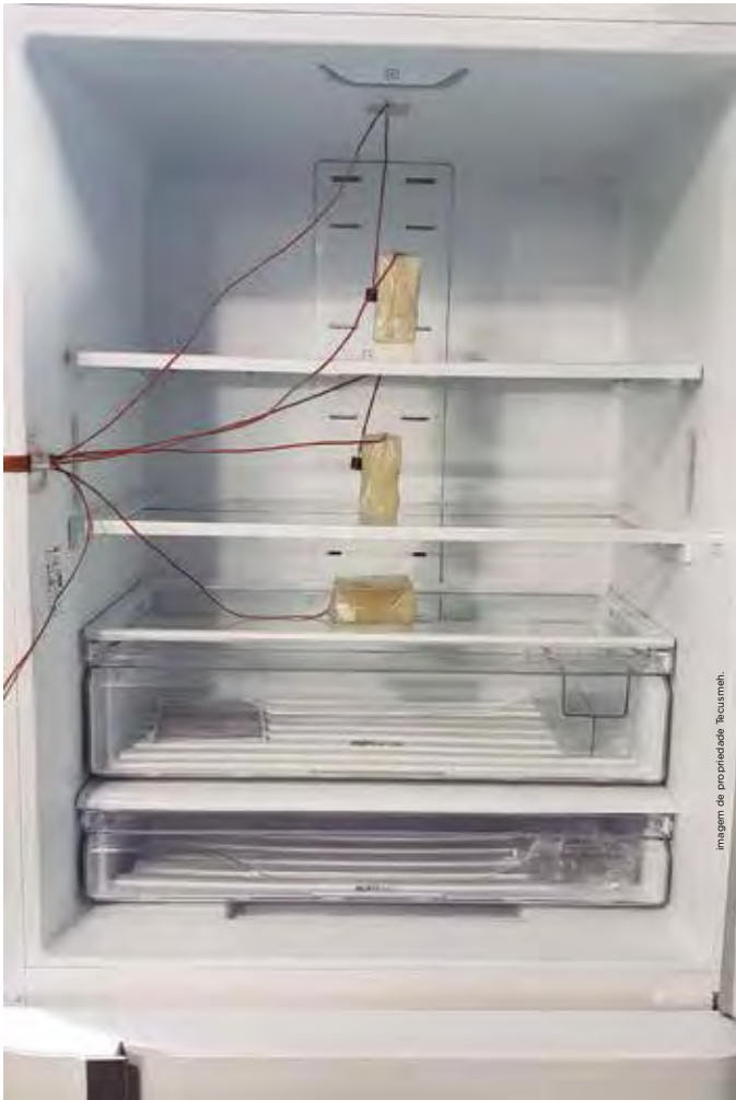
Duplex refrigerator fresh food compartment loaded with three monitored loads for carrying out storage and pull-down tests.
