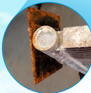
Salt Spray test in the Tecumseh lab in Brazil
