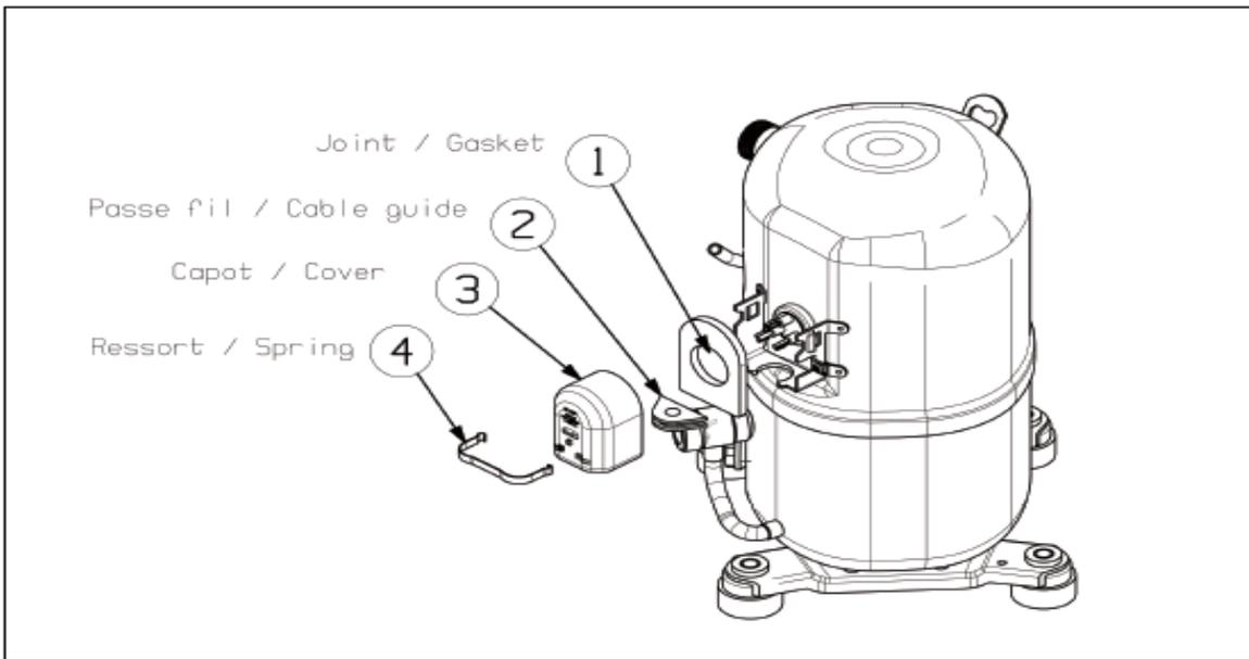
Assembly drawing for Protective cover for FH² Compressors
