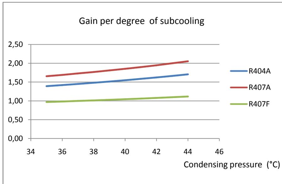
Curves are plotted at saturated pressures  $T_o/T_c = -10/45^\circ\text{C}$ , Dew /Dew.
